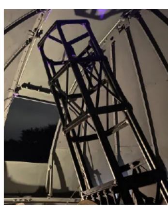
The Astronomical Society's 18" Newtonian telescope
